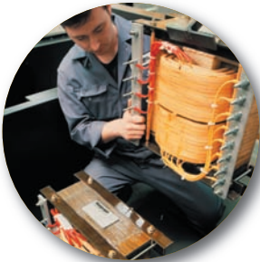
In house manufactured transformers
