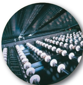
2 UV lamps above and 1 below peek wheels
