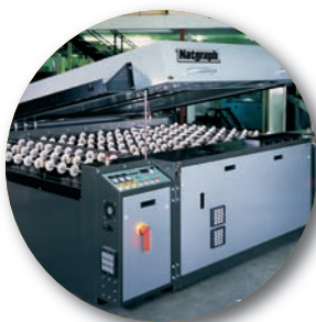
3 lamp UV Glass Dryer with driven peek wheels
