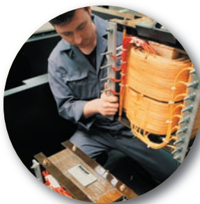
In-house manufactured transformers
