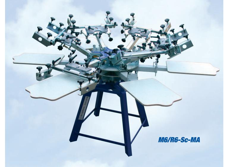
4- or 6-colour carousel, delivered either with 4 or 6 rotating printing pallets or with 1 stationary non rotating pallet.
